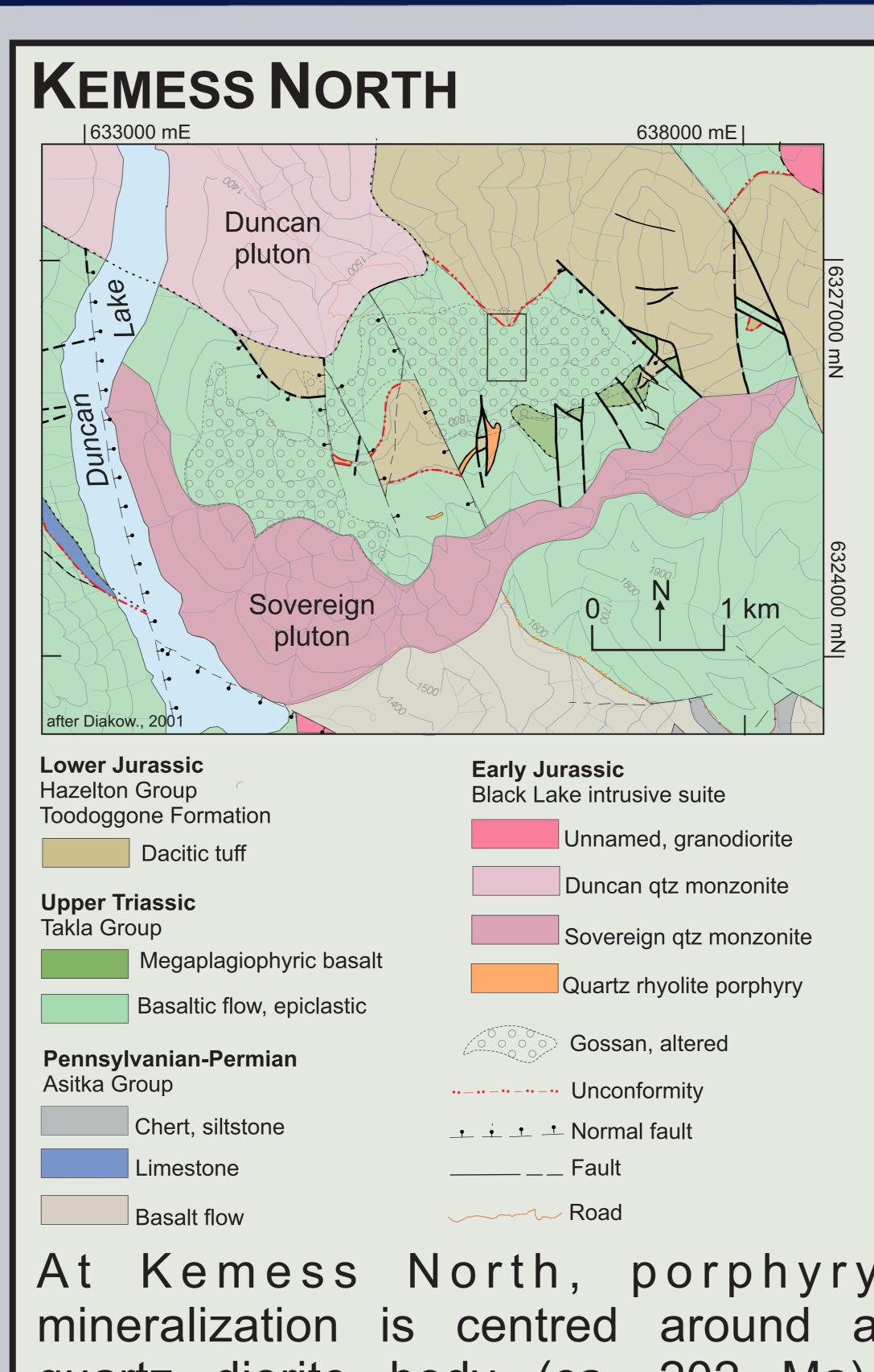
mineralization is centred around a quartz diorite body (ca. 202 Ma Associated phyllic-type alteration and is Sericite characterized by very fine-grained is characterized by quartz-magnetite rich to Fe-Mg rich with no obvious trends. chalcopyrite ratio.
